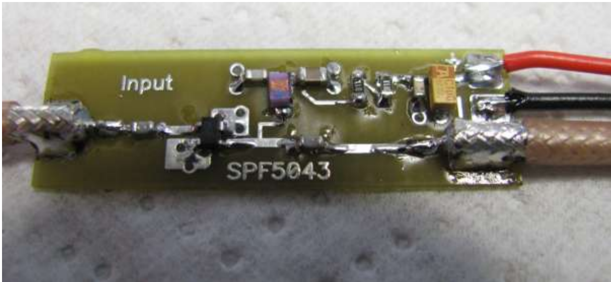
Photo 1 Assembled SPF5043Z amplifier. Note that after kit serial 125 0603 size a 100nH inductor is being supplied for the L1 position
