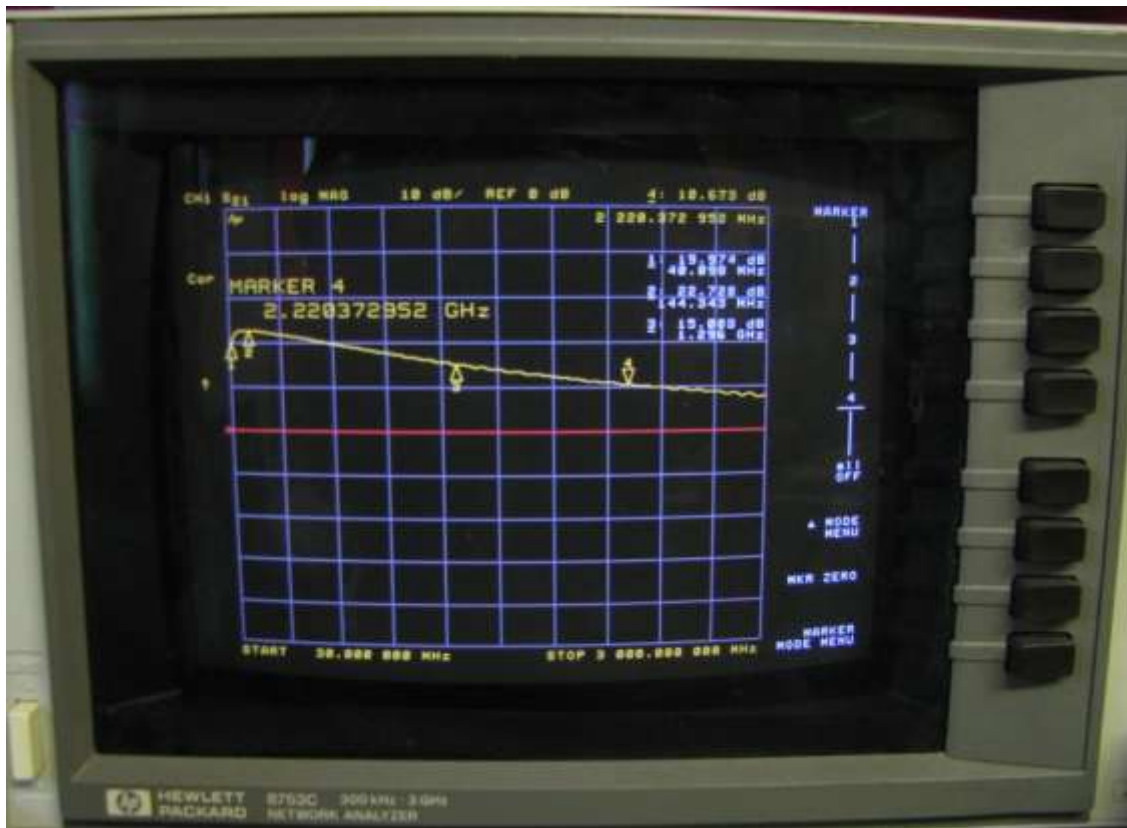
Photo 2 Insertion gain from 30MHz to 3GHz. Markers at 40, 144, 432 and 1296MHz. The gain is 20dB at 40MHz, 22.7dB at 144MHz, 15dB at 1296MHz and 10.6dB at 2.3GHz. The red line is 0dB gain. The yellow line indicates the gain at 10dB / division. The input power level was set at -20dBm.
