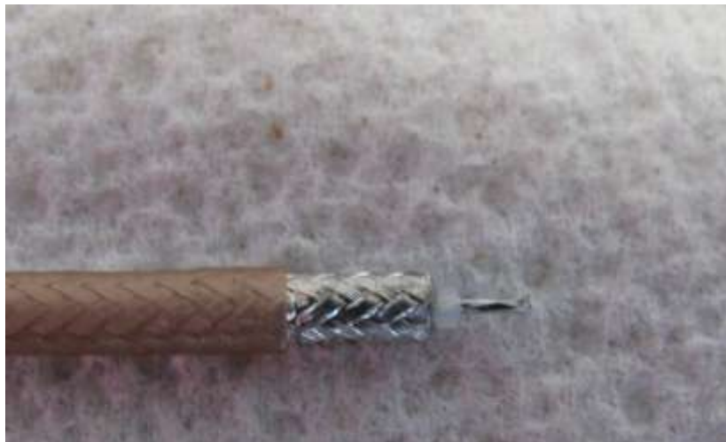
Fig 4 RG316 Cable preparation, final stage
