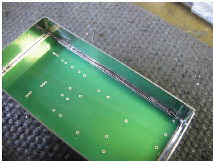
Fig 12 seam soldering the PCB into the box
