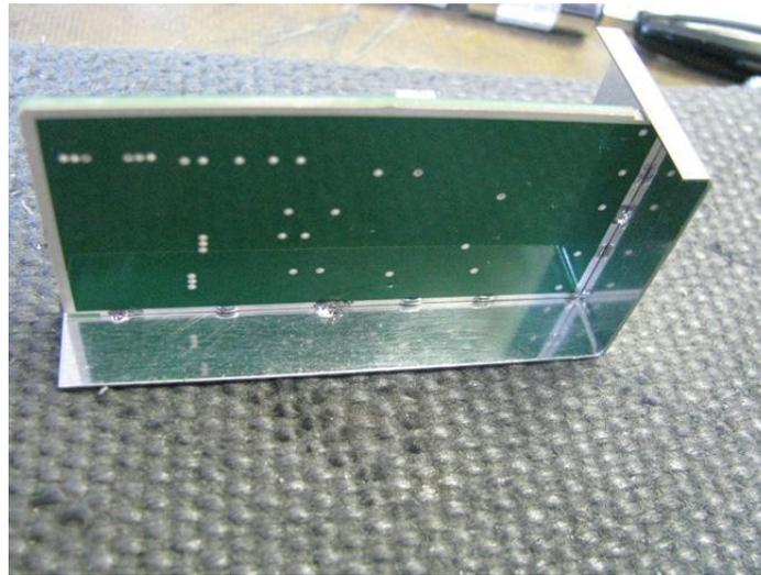
Fig 10 soldering the PCB into the box
