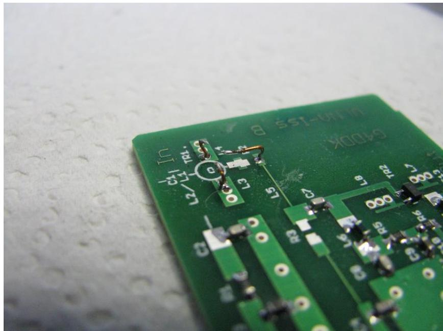
Fig 6 source wires in place plus drain wire
