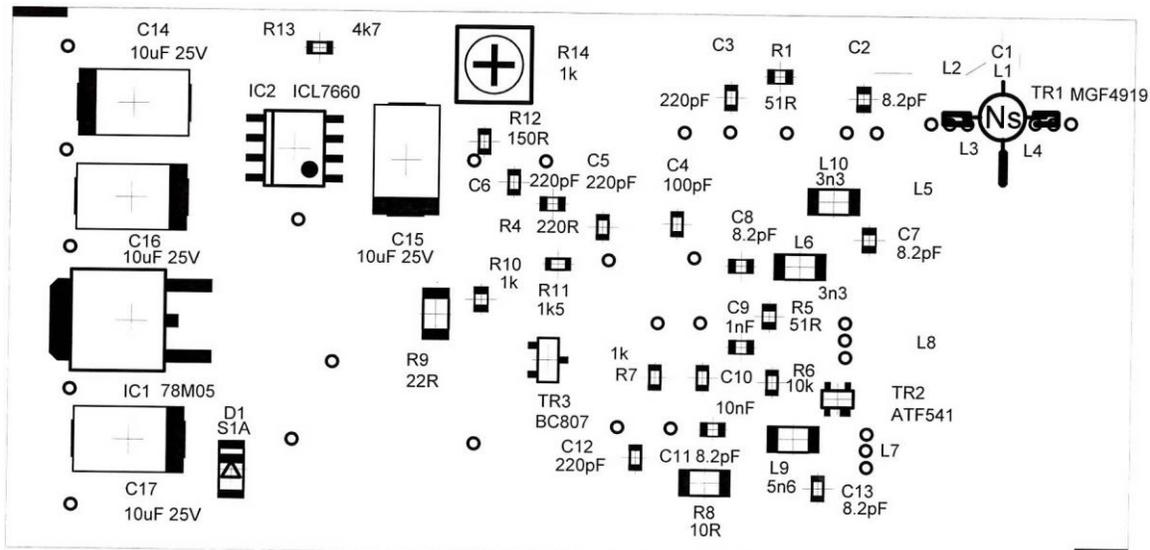
Fig 4 Component overlay (Component values shown for VLNA23)
